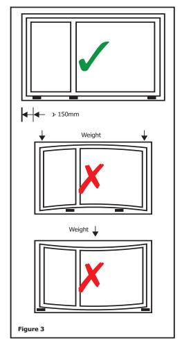
Support for the frame should prevent distortion and avoid damaging any protection or finish.
