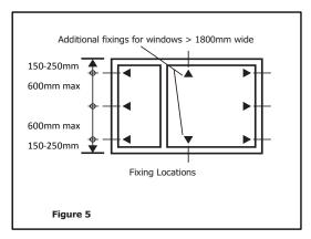
Special requirements may be necessary when fixing windows into preformed openings. Unless internally fitted fixing clips are used (*Figure 6*) you will have to fix through the frame. Choose unobtrusive locations.
